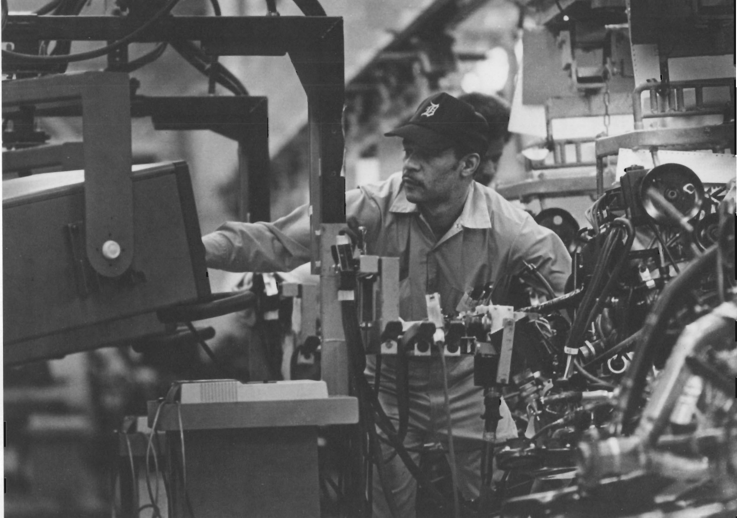
Hewlett-Packard computers guide a GM technician through an electronic battery of tests to measure engine speed, manifold pressure, air flow and temperature settings for a 3-liter Cadillac engine. A finished 1987 Cadillac from Hamtramck has five on-board computers.
