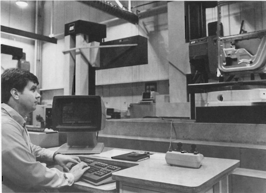
An HP 1000 computer controls a coordinate measuring machine that fits a car door to its frame. The electronic equipment helps keep tolerances within a millimeter of perfection.
